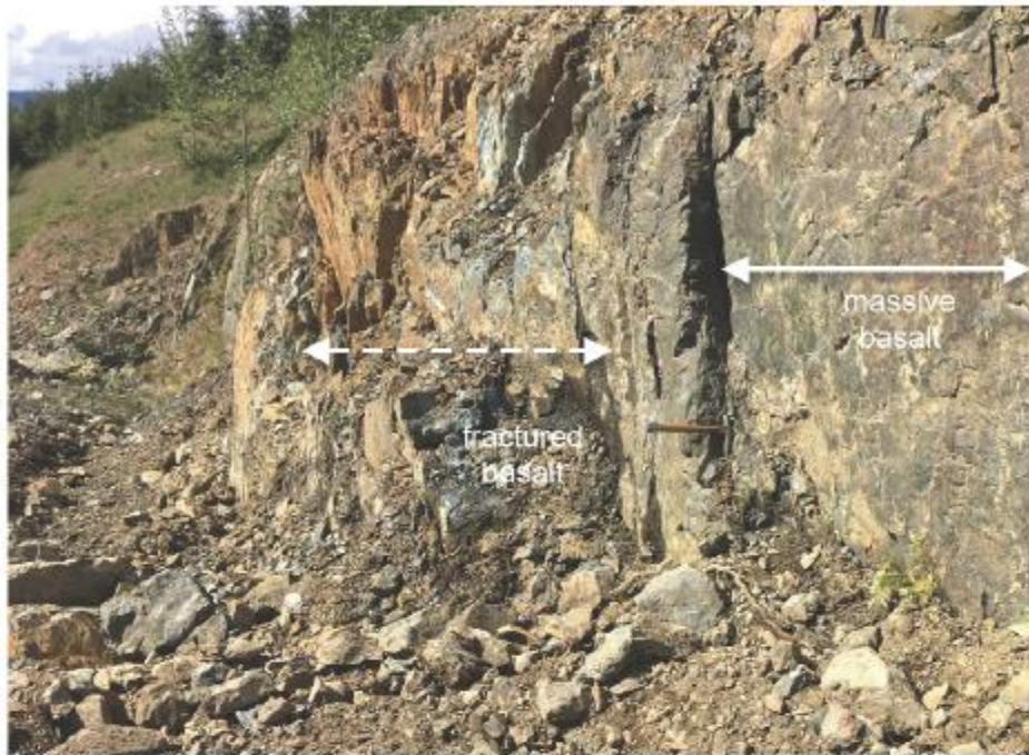
Photo 1. Outcrop of fractured basalt looking northwesterly along north side of Aythree Way extension near entrance to Otter Point Estates, April 25, 2021.
