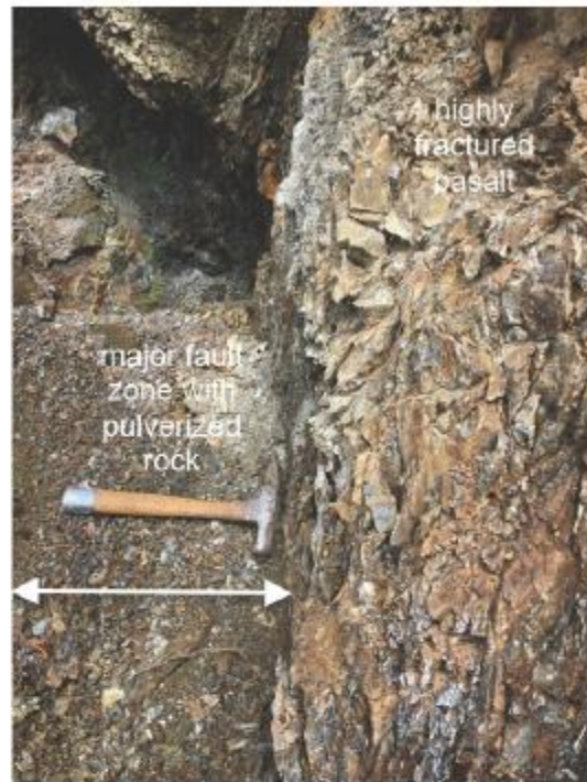
Photo 3. East side of large near vertical fault zone with soft pulverized rock looking northerly near western boundary of proposed Lot 2, April 25, 2021.
