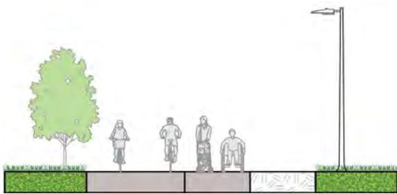
Separated bike path and walkway, with an adjacent soft surface trail.
