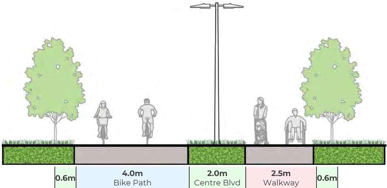
Another separated pathway option is considered that includes a 4.0m bike path and a 2.5m walkway (as above), but with a 2.0m wide centre boulevard space. The bike path has a dashed yellow centre line and pavement markings indicating the intended travel direction.
