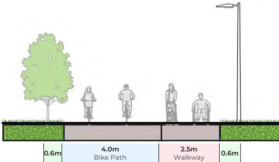
A separated pathway option is considered that includes a 4.0m bike path and a 2.5m walkway. The treatment includes a solid white line separating the cyclist and pedestrian facilities, as well as dashed yellow markings on the bike path and pavement markings indicating the intended user and travel direction in each space.
