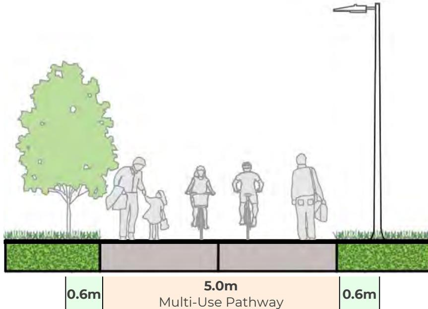
A 5.0m wide multi-use pathway option represents a similar configuration to the current trail condition, but with widening of up to 2.0m along its length. The treatment includes two 2.5m multi-user lanes with a dashed yellow centre line that allows for passing.
