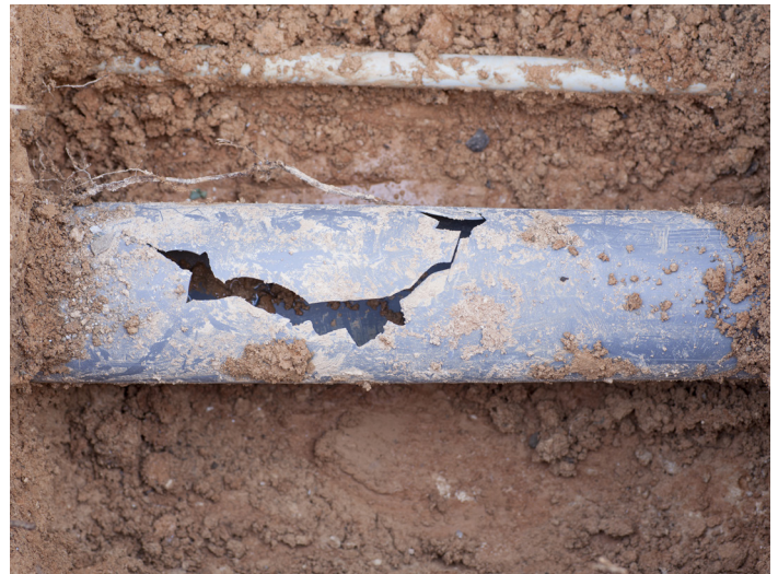
Cracks, breaks, leaks at joints or collapse from shifting ground or deteriorating material
