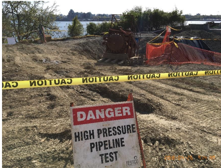
Figure 8 – Hydrostatic test in progress – the test passed.
