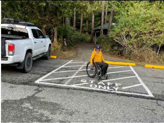
Staff Only Parking in What Should be a No Parking Area Between to Accessible Parking Stalls
