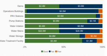
Overall condition rating of the asset classes is based on remaining expected service life. Replacement values are shown in relation to the condition rating.
