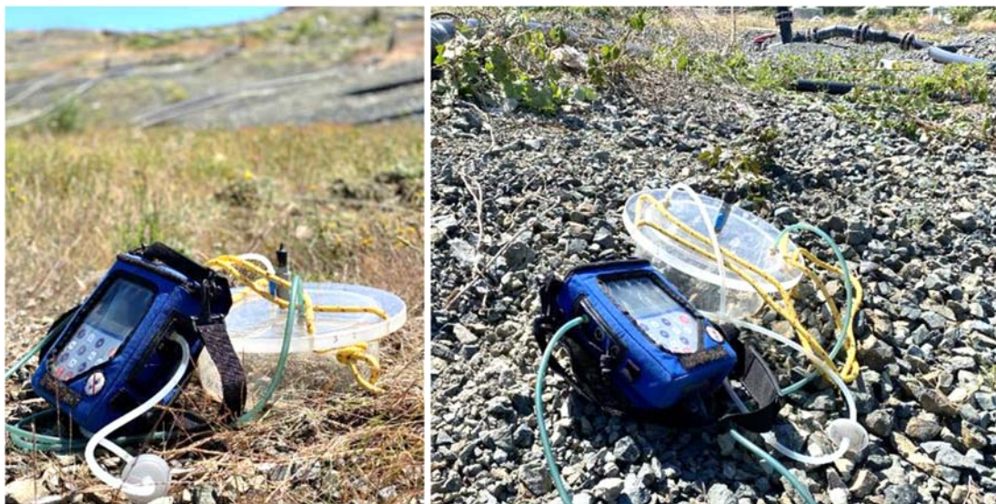
Photo 4.10a & 4.8b - Flux Chamber Measurement at Hartland Landfill
