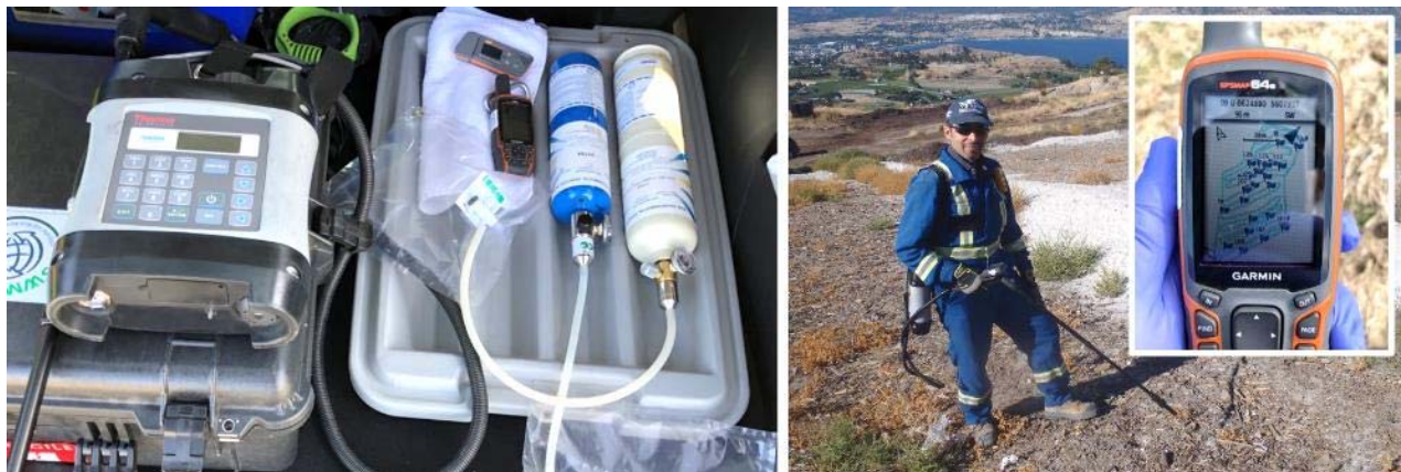
Photo 3.1a & 3.1b - Surface Methane Concentration Scan Using a Portable FID Instrument
