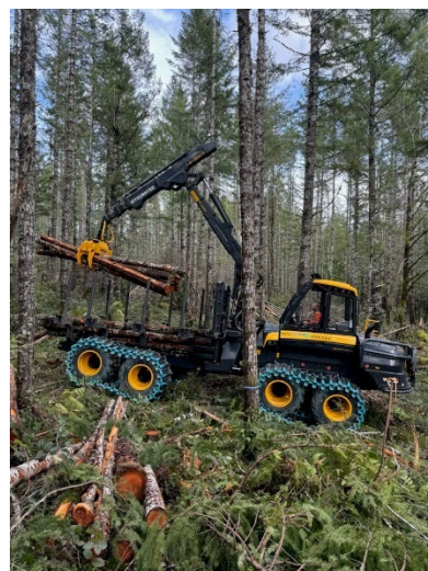
View of the narrow forwarder loading into its bunk with low ground pressure tracks and long boom reach.
